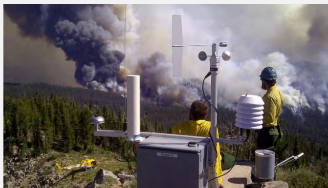
Remote Area Weather stations provide essential weather data used to understand trends in wildfire risk
